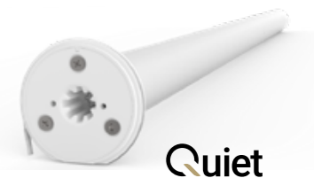
Automate Wire-Free Li-ion Zero Q2 5V, 2.0Nm, Ø28mm, 20-28RPM, 649mm long
