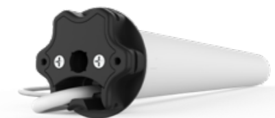
Automate AX50 240V, 50Nm, Ø45mm, 12RPM, 676mm long
