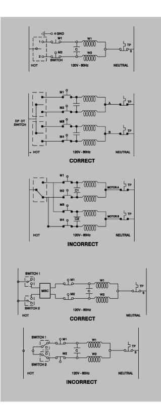
Because of the type of motor (Asynchronous with built-in capacitor) and the built-in limit switches, it is important to follow two important recommendations to assure proper operation of the motorized systems - Automate Operators are not universal motors.
