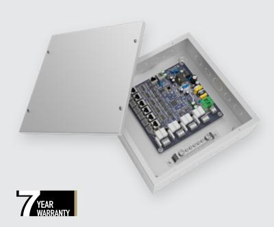
The 4-Channel Motor Controller is a standalone unit that controls up to four Mechanical Limit motors all on one switch, individual switches, or even dry contact closure devices. By default, the controller has four intermediate positions (20%, 40%,60%, and 80%) to provide precise control of each shade.
