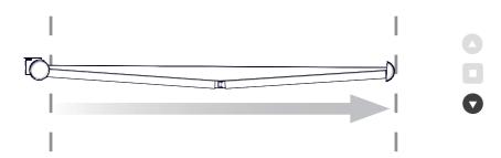
And **UP** on the remote CLOSES the Awning (awning moves in an inward direction). E.g.
