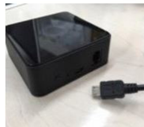
3. INSERT THE MICRO USB END OF THE POWER CORD (LONG OR SHORT) INTO THE WI-FI BRIDGE.
